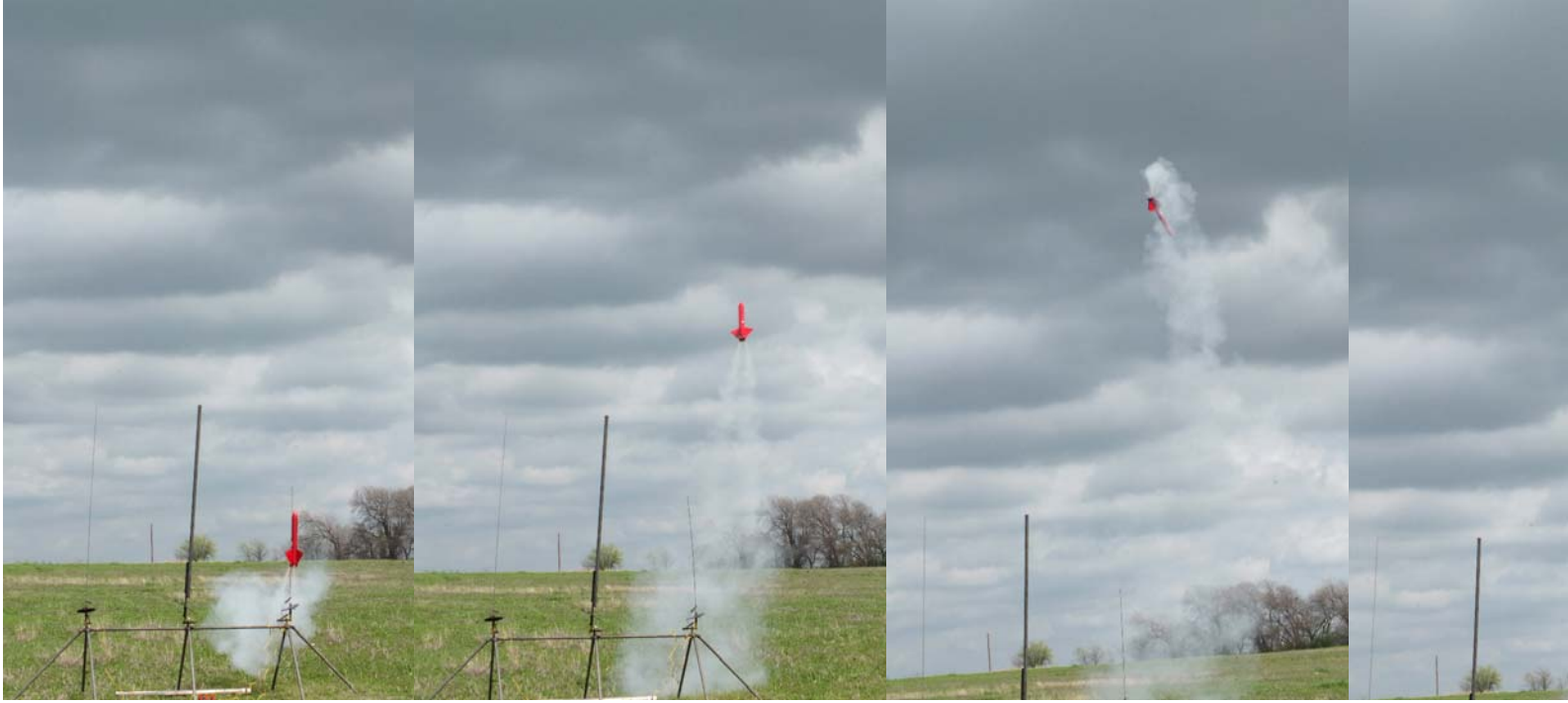
Figure 5 - What happens when you light 2 motors of a 4 motor canted cluster (in spectacular PANOMANIA!!!!) Briggs photo
